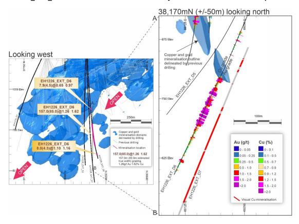
Figure 4: Section 38,170mN (+/-50m) looking north showing the mineralisation intersected in EH1226\_EXT\_D6 50m north of EH1226\_EXT\_D3. Visual Cu estimate from EH1226\_EXT\_D7 shown in red which we expect will extend mineralisation down dip. EH1226\_EXT\_D5 awaiting results
