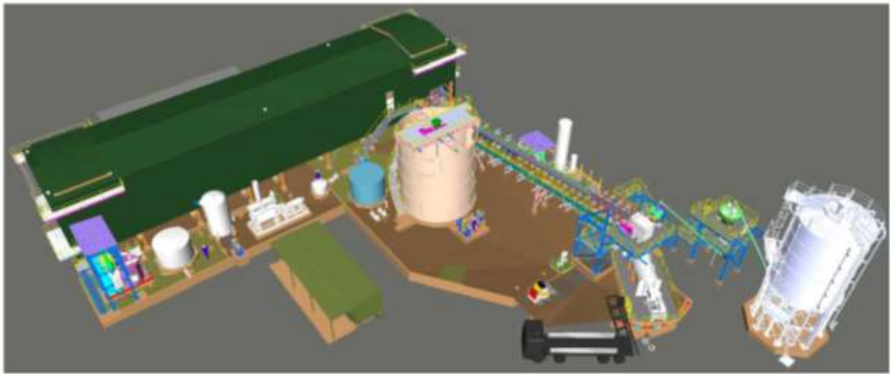
Figure 3.4 Paste fill plant general arrangement isometric view
