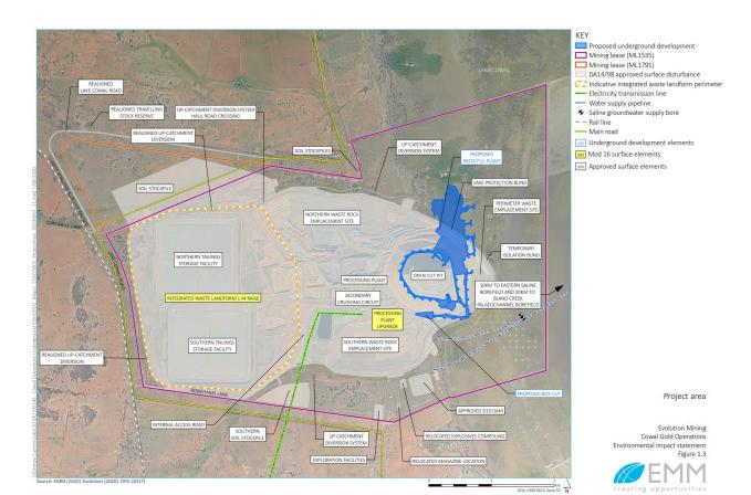
**Figure 3 Underground Development footprint layout**
