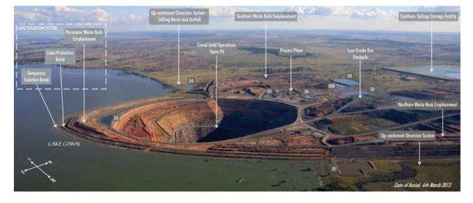
Figure 2 Key infrastructure and footprint of current mine operations
