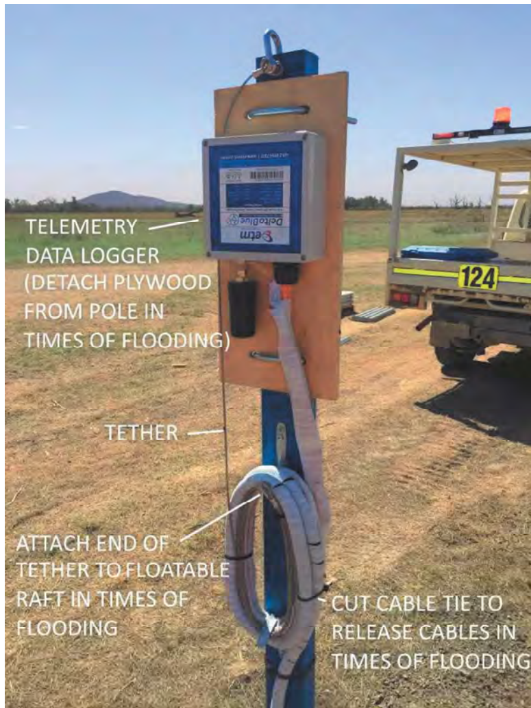
Figure 7: Telemetry installation
