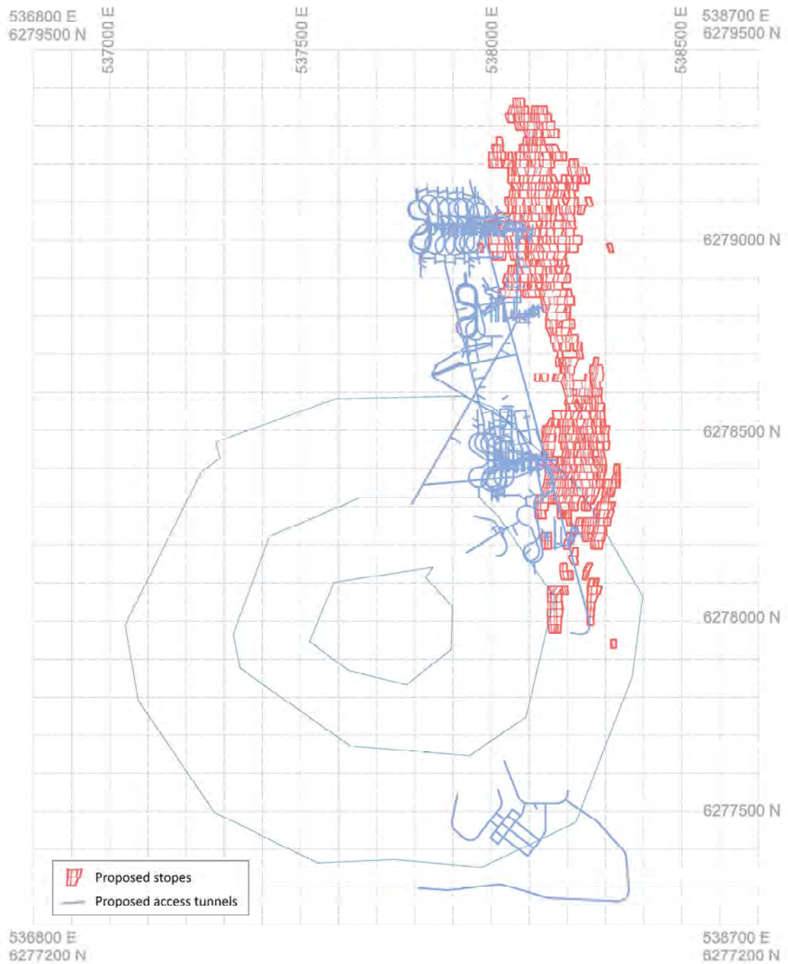
Figure 7-5: Stopes and access tunnels - plan view (m MGA Zone 55)
