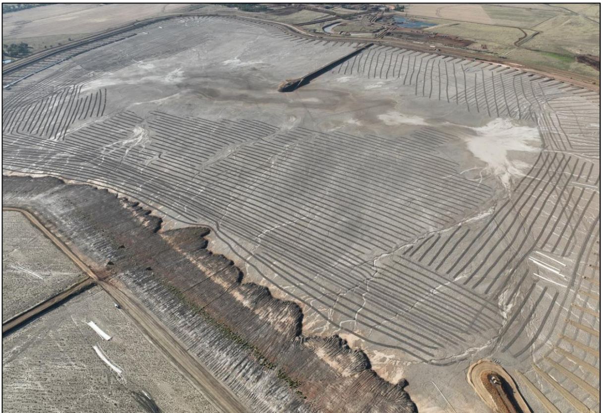
Figure 14 Ripping undertaken on Rosedale TSF for dust control
