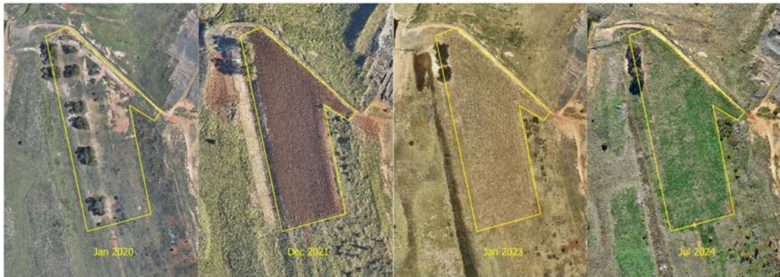
Figure 30 E22 waste rock batter rehabilitation repairs from 2020 to 2024
