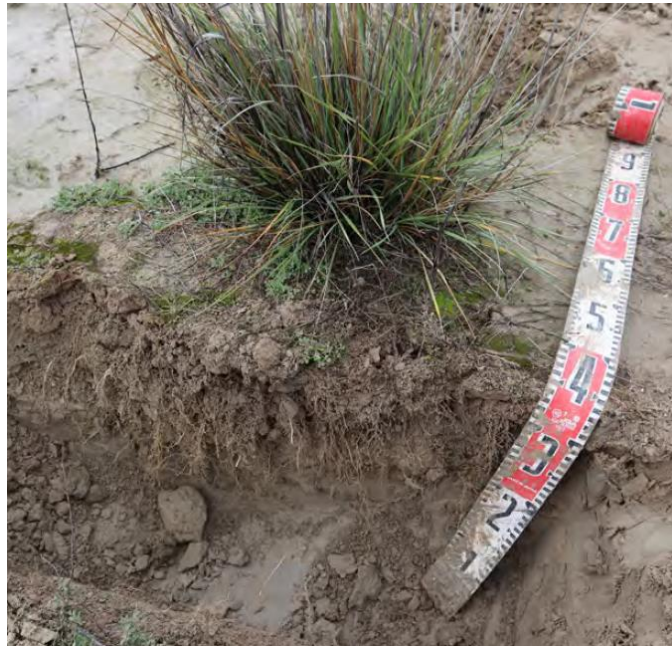
Figure 34 Perennial grass rooting depth in TSF2 tailings profile
