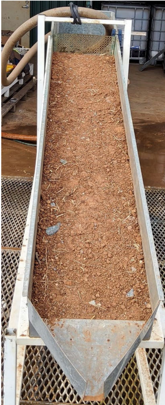
Photograph D3: Soil-rock matrix prior to being subjected to simulated overland flow.
