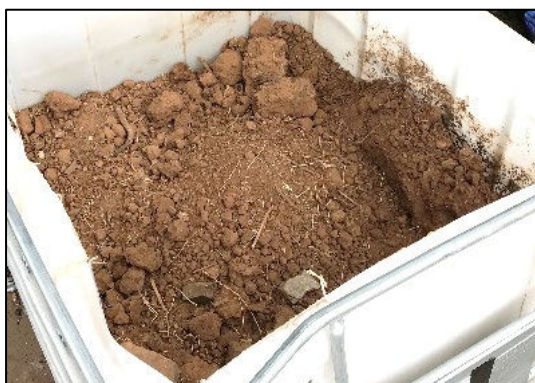
Photograph 1: Bulk sample of Soil-Rock Matrix Upper Layer.
