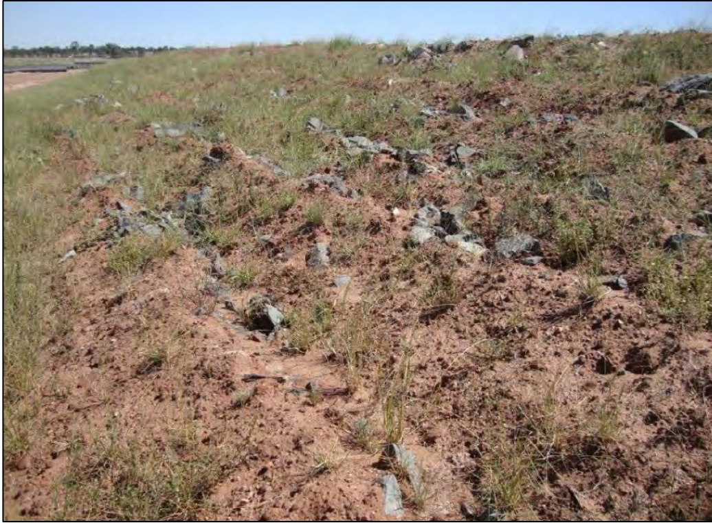
Photograph 2: CGO soil-rock matrix cover system with mounding formed by cross ripping (Photo courtesy of Donna Johnston, DnA Environmental).
