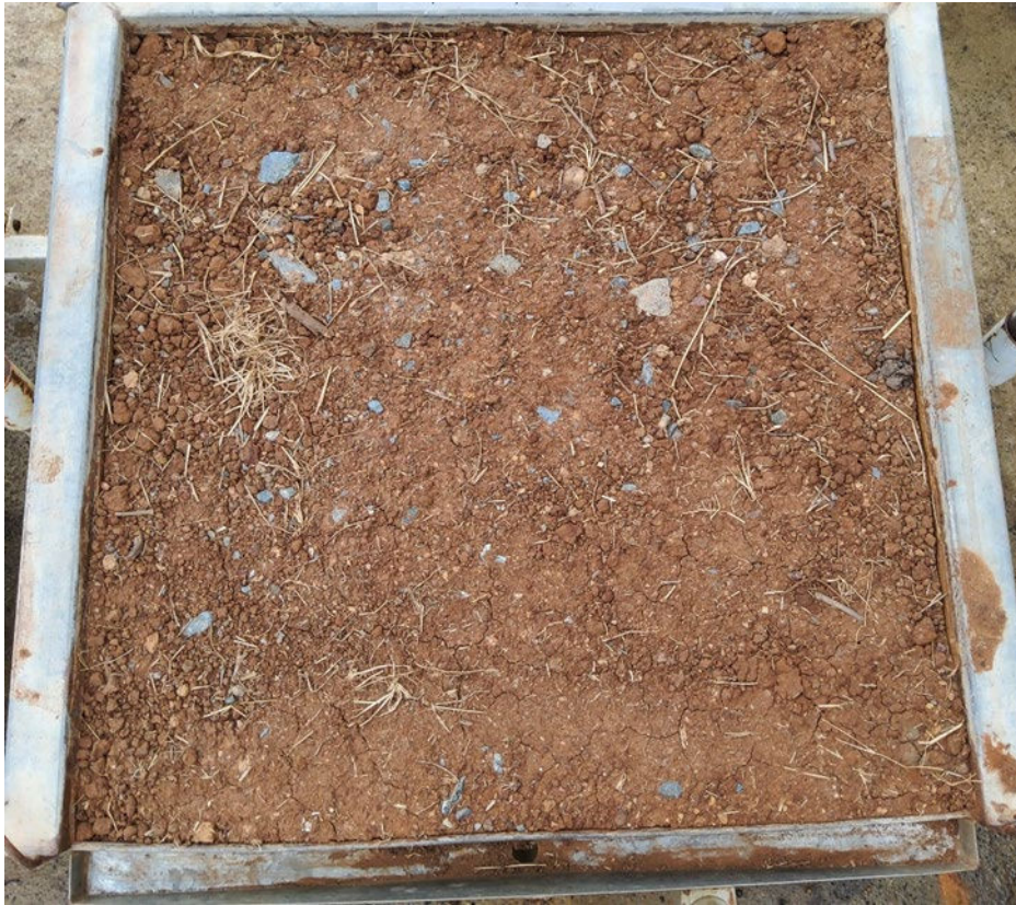
Photograph D1: Soil-Rock matrix prior to being subjected to simulated rainfall.
