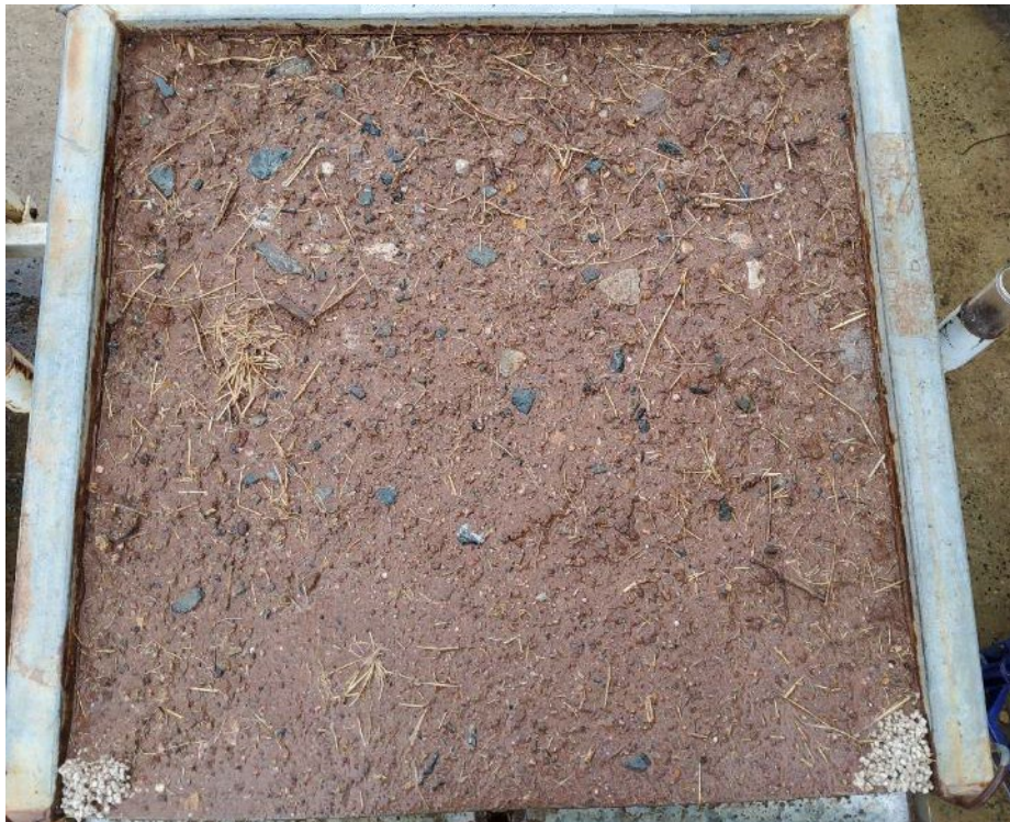
Photograph D2: Soil-rock Matrix after being subjected to simulated rainfall.
