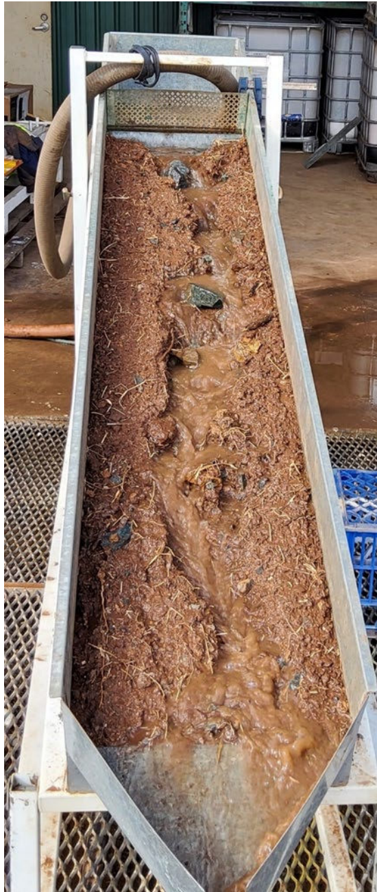
Photograph D4: Soil-rock matrix undergoing simulated overland flow testing.
