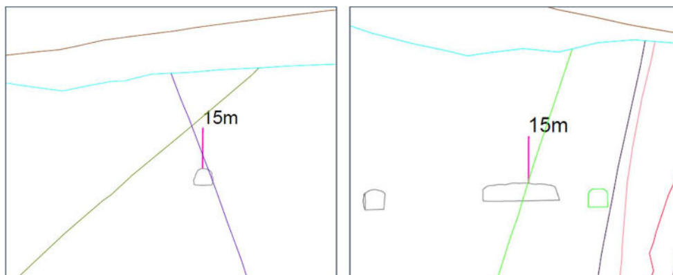
Figure 11. Section views of 15m extensometers to be installed in the WAR_1050_DD_N (left) and the WAR_1057_ACC (right).
