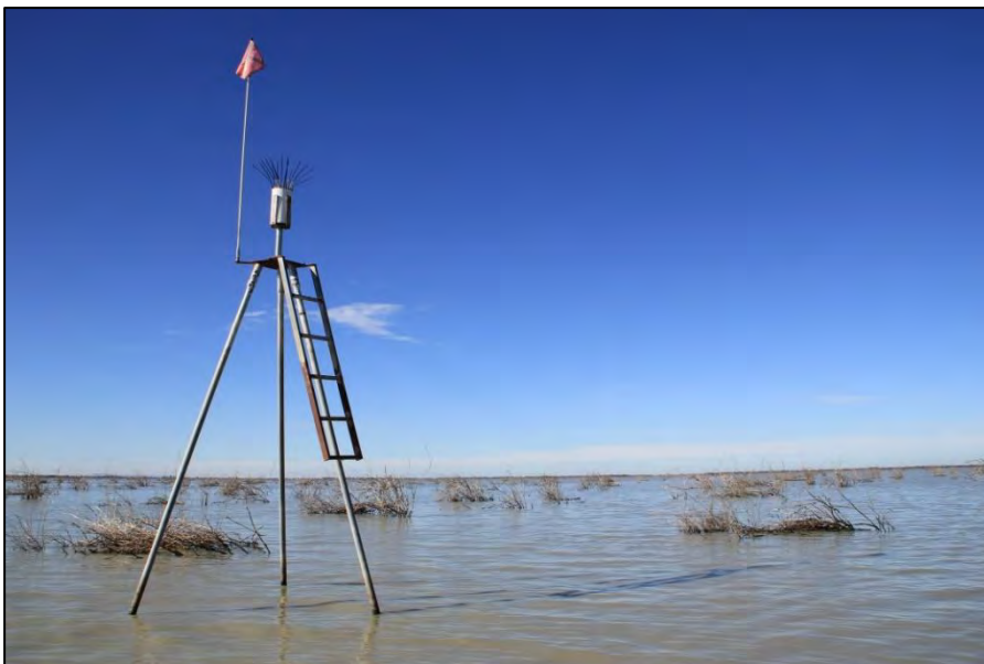
Plate 1: Elevated Depositional Dust Gauge within Lake Cowal
