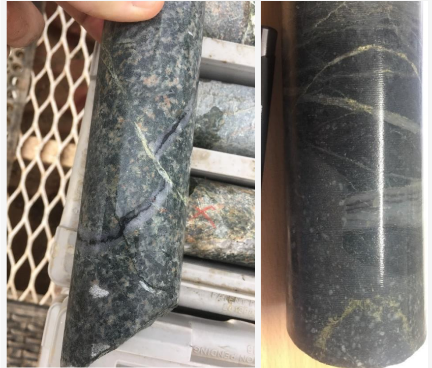
Chalcopyrite veins cutting magnetite veins in core from recent drilling at E41 West
