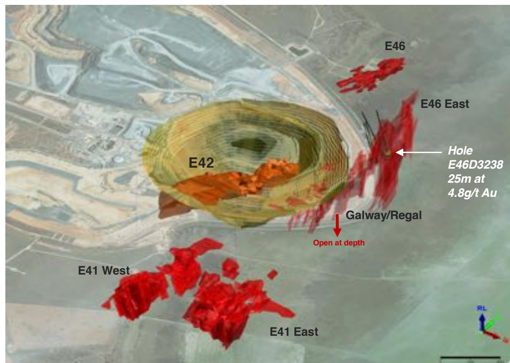
Cowal gold mineralisation, recent drilling and E42 open pit outline
