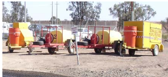
CGP fire water tankers and spill response units.
