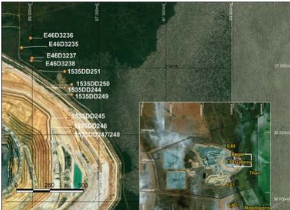
Cowal drill hole location plan showing drill hole traces of reported resource definition drilling
