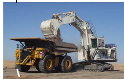
Plate 6: Leibherr R994 backhoe and Cat 789C dump truck in the pit – 06/05
