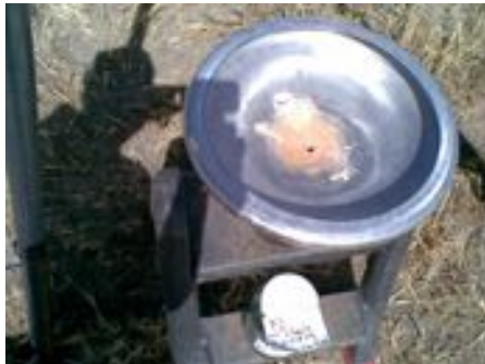
Plate 7: 'Frisbee' (directional dust deposition gauges)
