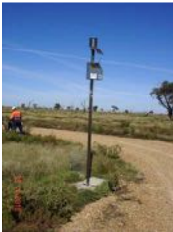
Blast monitor (BM04.1) with new track for all weather access and safety.
