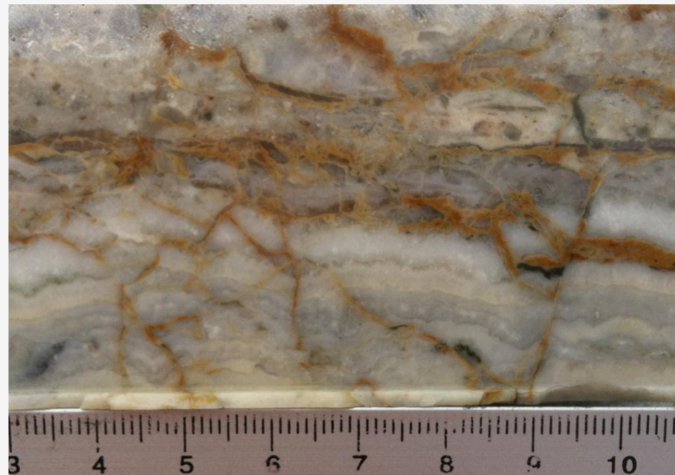
Camembert prospect: Epithermal textured - multiple crustiform & colloform banding and breccia events with adularia, chlorite and sulphosalt banding in JMRD3973W1 at 383.5m
