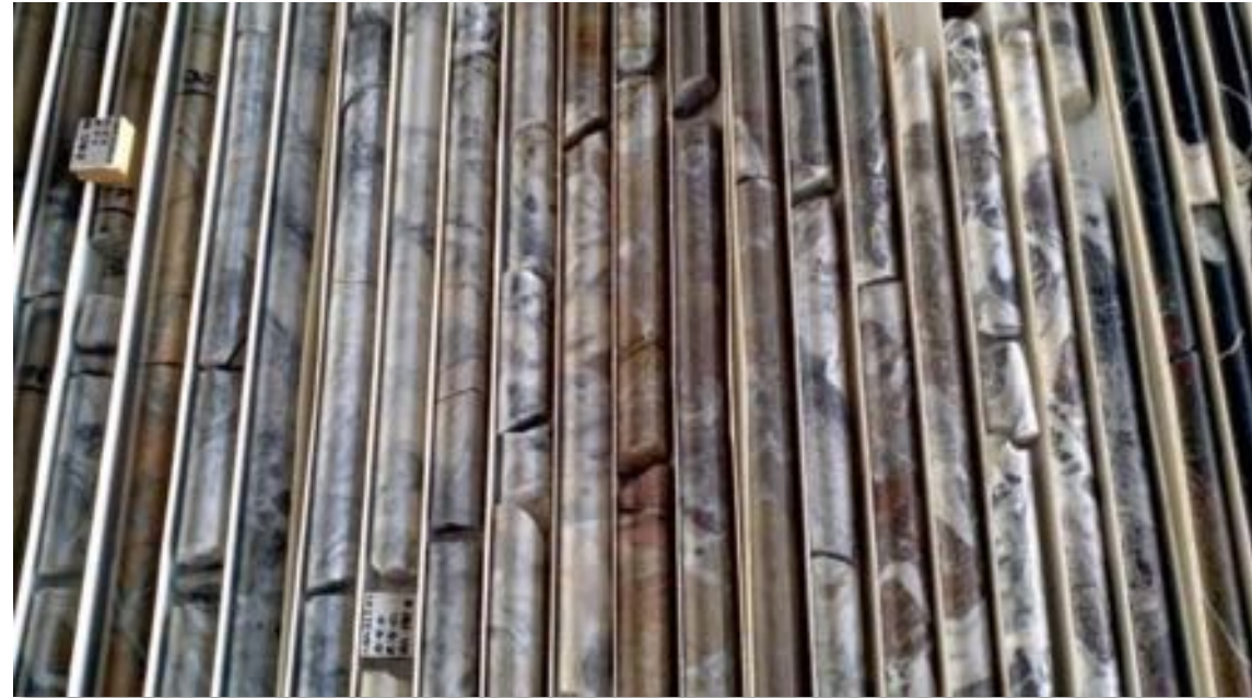
Drill core intersecting Imperial lode at Cracow (CBK353W1)
